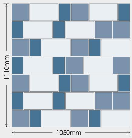
Each full crate is packed in layers - the pattern above shows one layer from a full crate. (10 layers per crate, total 420 pieces).
